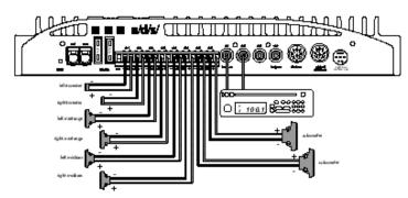
System 4 – The P850 is used in bridged 4-channel mode. Channels 1/2 and 3/4 are high-passed bridged-mono for front speakers. Channels 5/6 and 7/8 are low-passed summed bridged for sub-woofers. Front speaker level control is adjusted by the ch3/4 level control. Subwoofer level is controlled by the ch5/6 level control. the P840.2 is configured for 2-channel input.
